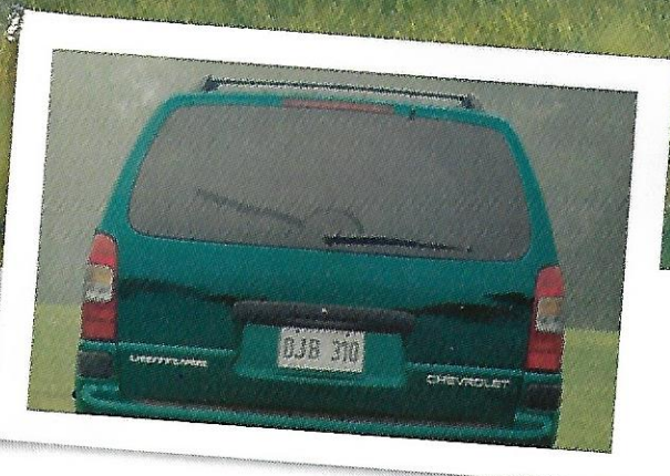
Liftgate With Wiper/Washer. Mounted in the center of the liftgate glass to eliminate blind spots, the Venture rear wiper/washer provides a 177-degree sweep. That ensures excellent visibility, which is important for safe driving.
