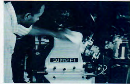
The optional 3.1 Liter V6 with Multi-Port Fuel Injection gives Corsica exceptional performance. Horsepower is 140 at 4200 RPM.
