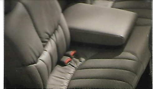
Rear-bench seat design with integral head restraints and center armrest.
