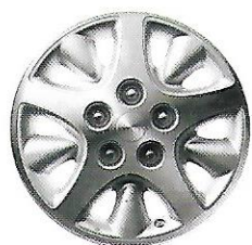
15-inch Quasar cast aluminum wheel (Set of four; available on Voyager SE and Grand Voyager SE)
