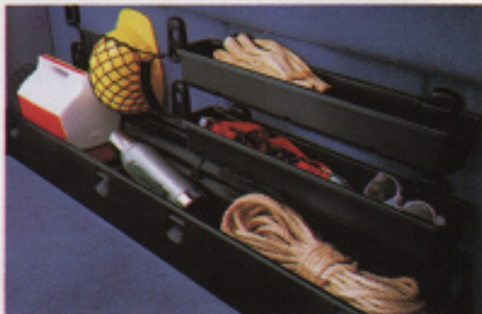
The Dodge Ram ST and Laramie SLT regular cab models have an exclusive behind-the-seat storage system which includes a cab-width floor tray, plus height-adjustable bins and cargo net.
