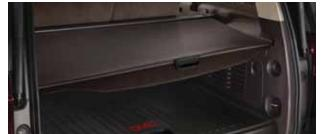
Cargo Security Shade Conceal your possessions in the cargo area of your Yukon with this retractable cargo shade. Tension-rod extensions allow for easy installation and removal.
