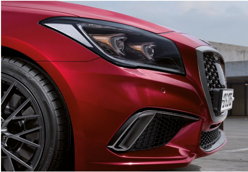
Full LED adaptive headlamps & Air curtains _ Copper chrome details on the headlamps convey a dynamic image. Vertical-type air curtains beneath the lamps reduce the aerodynamic drag of the vehicle.
