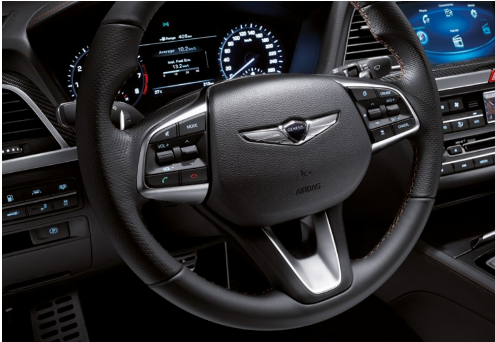
3-spoke steering wheel _ A 3-spoke steering wheel with a wider rim that optimizes the grip; and paddle shifters that were specifically designed for the sports model to improve driving maneuvers.
