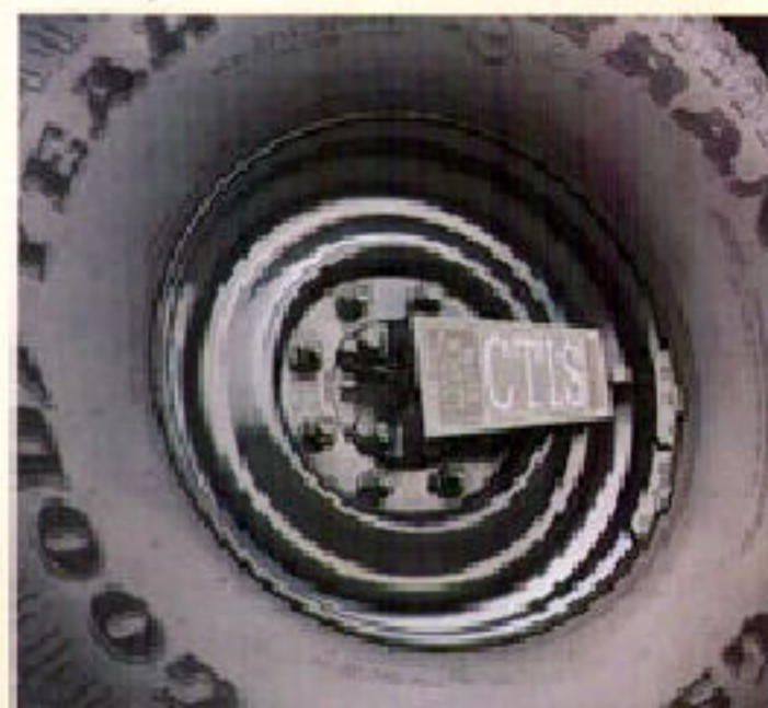
All 1997 Hummers have a lighter, one-piece heavy-duty wheel with runflat and beadlock capabilities.
