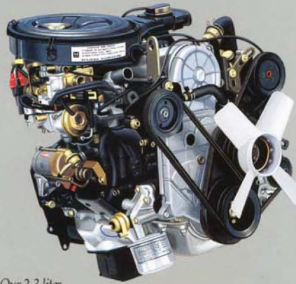
Our 2.3 liter gasoline engine pumps out 96 horses and 123 ft.-lbs. of torque.
