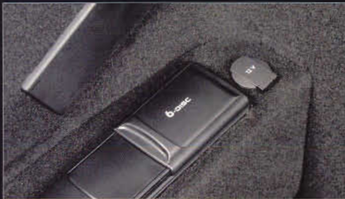
Power socket in trunk
