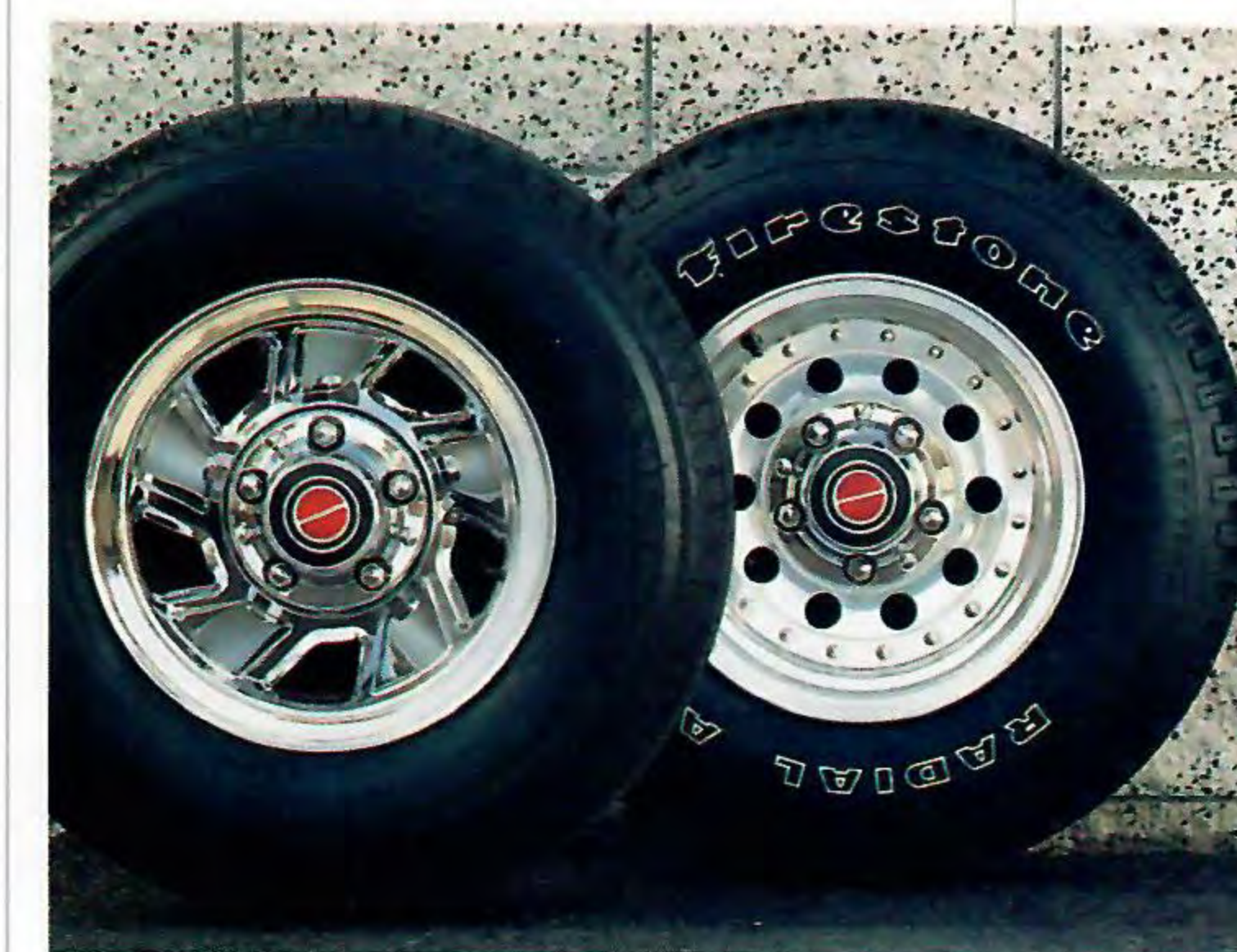
Wheel options include new 15" x 7.5" chrome-styled steel wheels on all models except the "Nite" truck. Forged aluminum deep-dish wheels, shown right with P265/75Rx15 OWL tires (late availability) are standard on Eddie Bauer and the "Nite" truck; optional on XLT and Custom.
