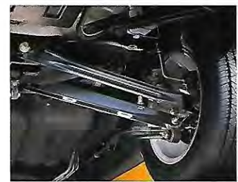
Independent rear Quadralink suspension system is a rather advanced system. We'll try to explain it. Each wheel can independently react to bumps in the road, moving both upwards and rearwards to absorb and reduce impact harshness. In plain English: This car can handle.
