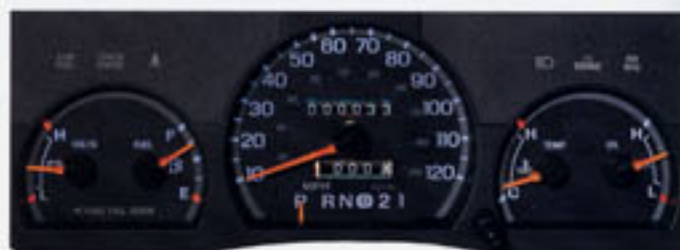
The analog instrument cluster includes battery charge, fuel level, engine temperature and oil pressure gauges.
