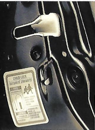
Childproof door locks can be engaged to prevent children from opening car doors from the interior.
