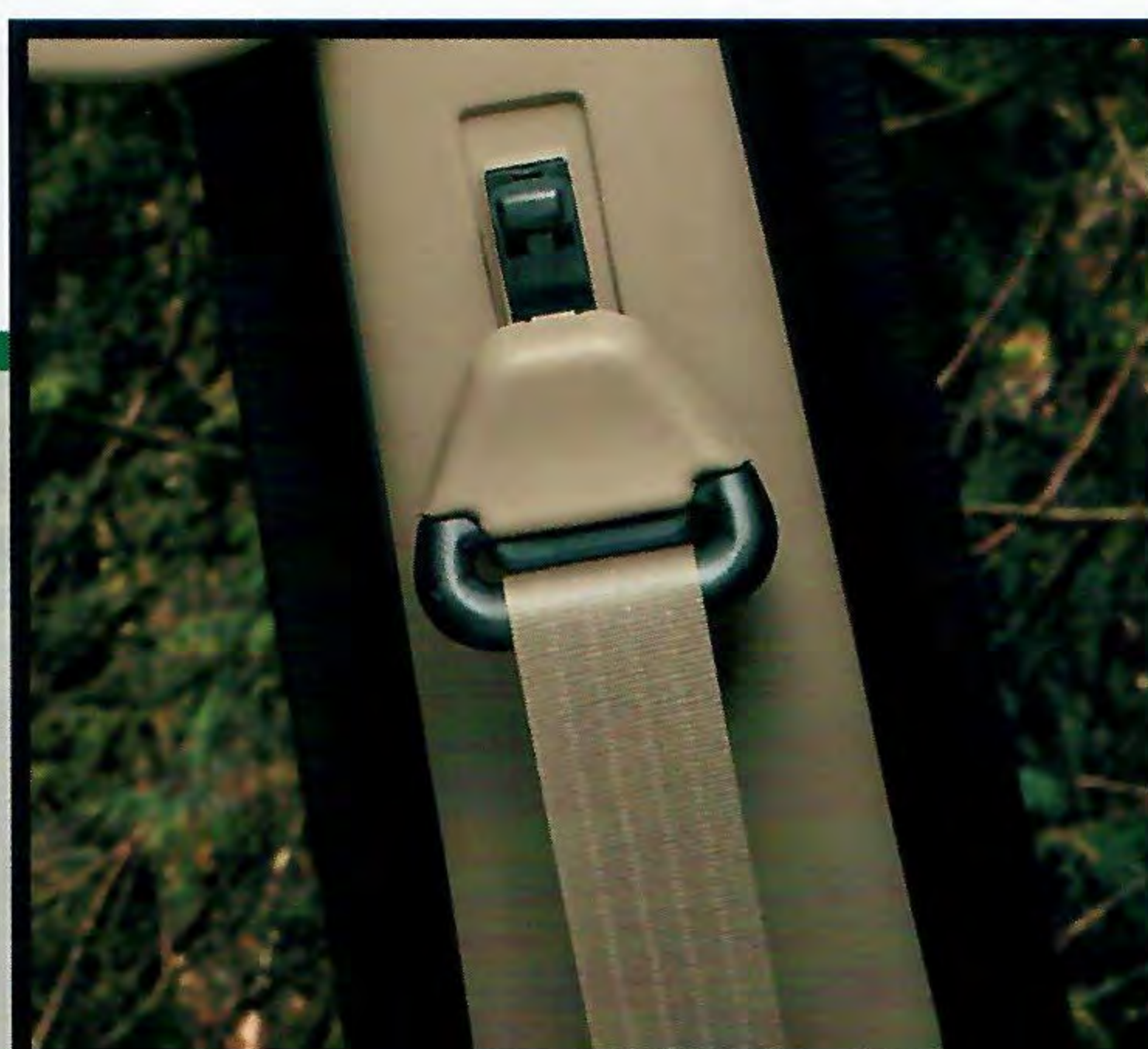
Adjustable harnesses. The height of the front and second-row seat shoulder harnesses can be adjusted to five different positions for individualized comfort.
