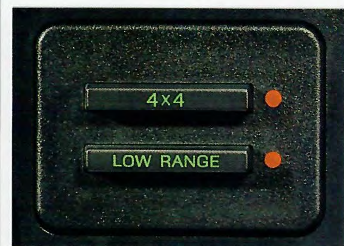
Push-button controls for the Touch Drive electric shift transfer case (standard in all 4x4s) are located on the instrument panel — a more convenient arrangement than the floor-mounted shift found in other 4x4 compact utility vehicles.
