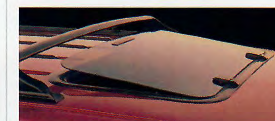
The tilt-up open air roof can be flipped open or removed. The roof rack (standard on Eddie Bauer) is also shown.
