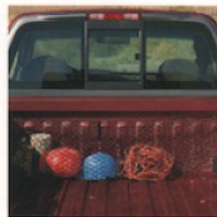
This cargo net secures items like tools and hard hats inside the pickup box.
