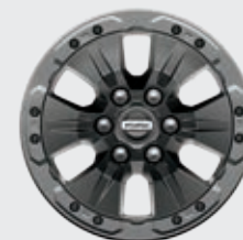
17" Forged Aluminum Bead-Lock Capable RAPTOR – Optional
