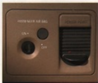
The passenger airbag deactivation switch must be used when a rear-facing child safety seat is employed (not available on Crew Cab).
