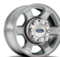
17" 6-Spoke Cast-Aluminum Standard: F-250/F-350 SRW
