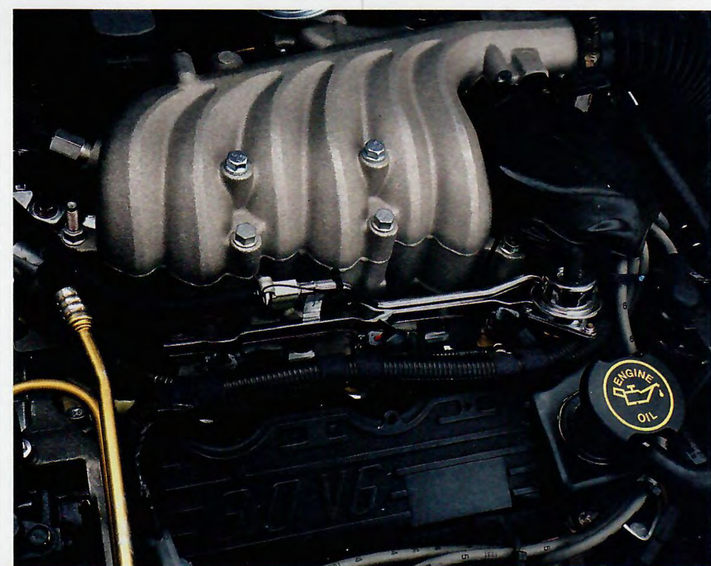
The Tempo GLS for 1992 is the most exciting Tempo sports sedan ever. It's powered by a 3.0L V-6 equipped with a computer-controlled, sequential electronic fuel-injection system. Its tuned intake runners are designed to balance high-end power and low-end torque.
