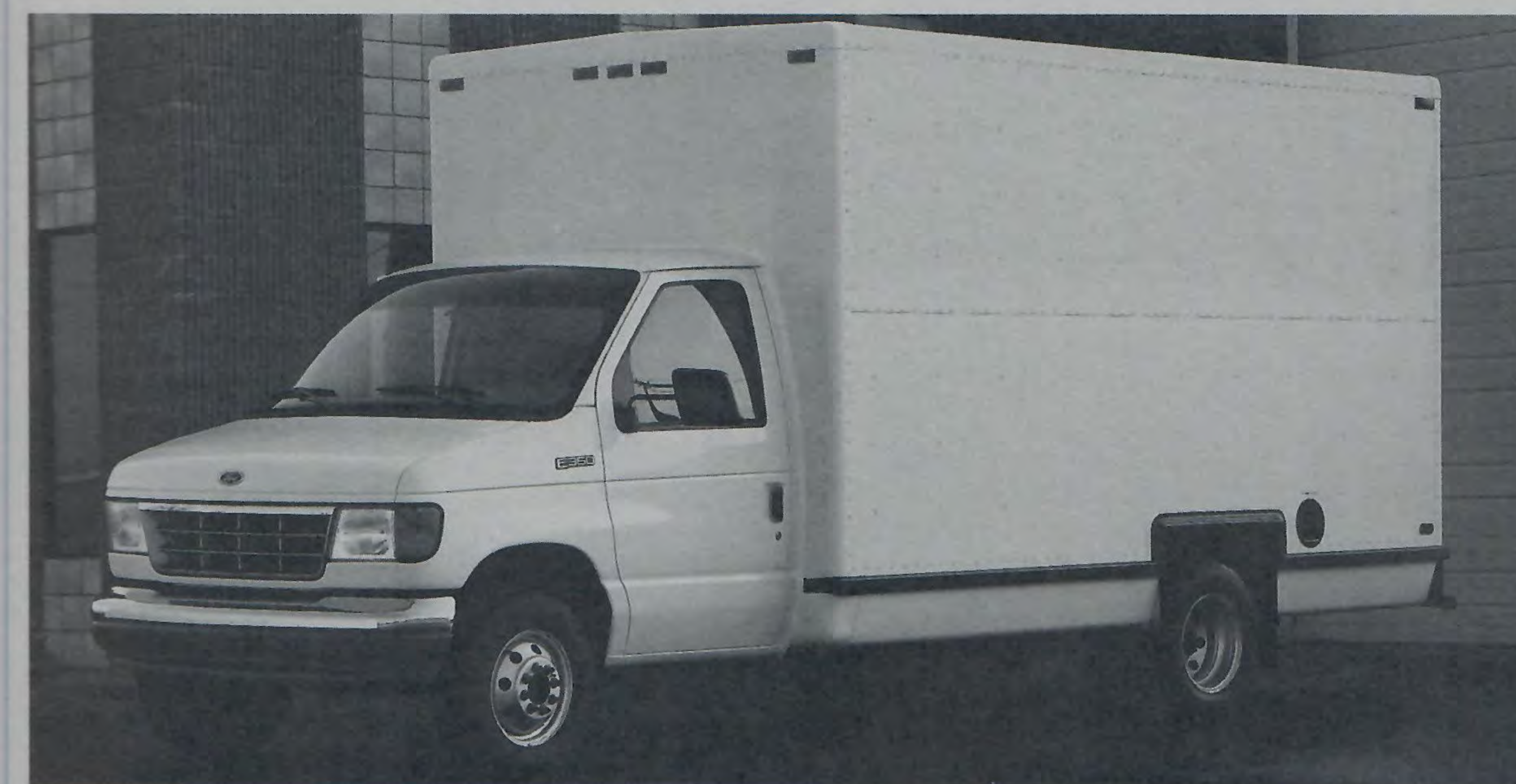
Left: The Econoline E-350 Commercial Cutaway features dual rear wheels and a payload capacity up to 5,985 lbs. (10,700-lb. GVWR).
