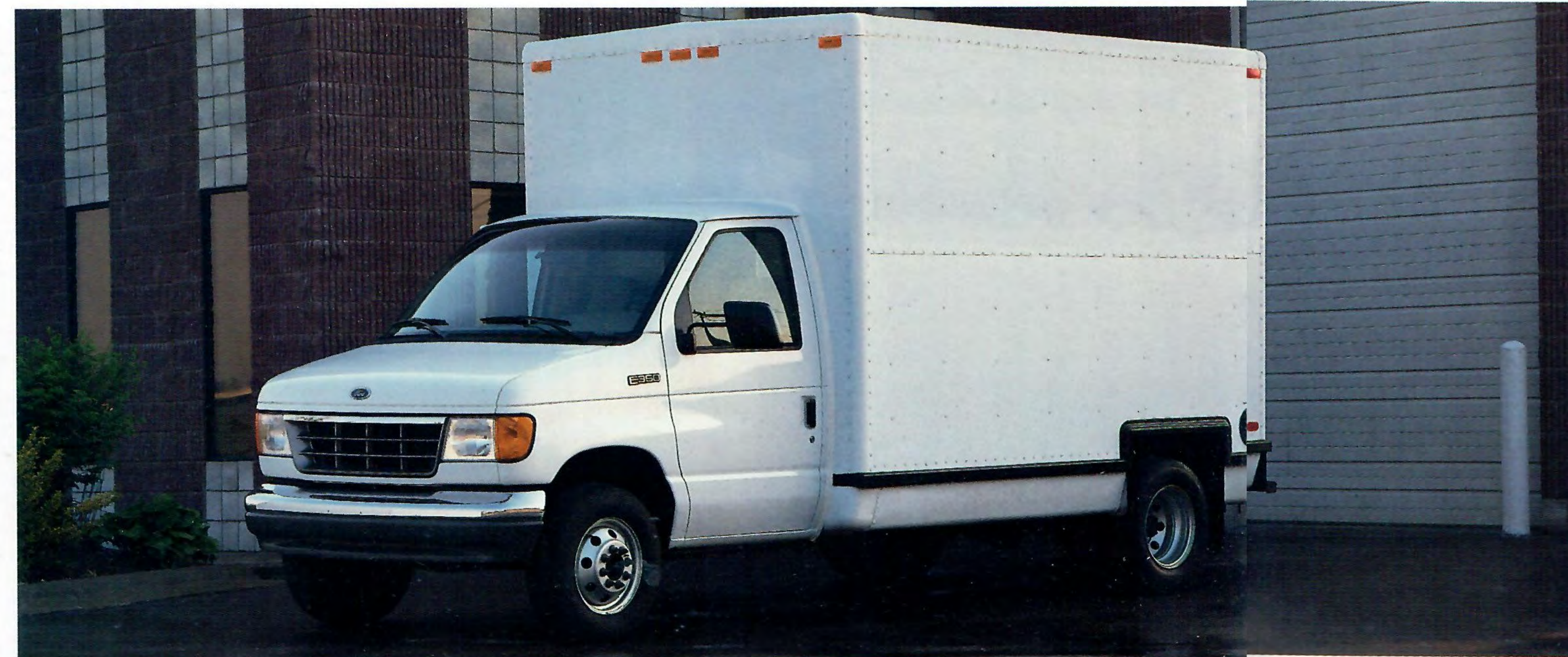
The Econoline Cutaway Chassis provides the frame and cab compartment preparatory to the installation of a custom cargo or RV body. See pages 16-17 for cutaway chassis information.
