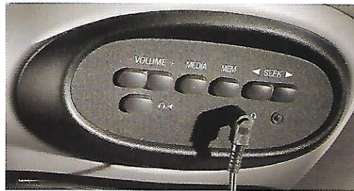
Equipped with rear seat audio controls, the Personal Audio System, a feature of the optional Premium AM/FM/cassette/single CD stereo, allows simultaneous listening of separate audio inputs. For example, rear passengers can listen through headsets (not included) to a CD, while front passengers listen to a cassette tape.
