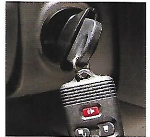
The SecuriLock™ Passive Anti-Theft System "interrogates" your encoded key, preventing would-be thieves from starting the engine.
