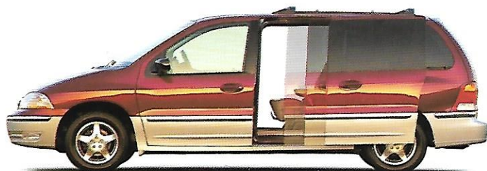
Optional driver-side and passenger-side power sliding doors can be activated from two interior push-button locations and a remote key fob.
