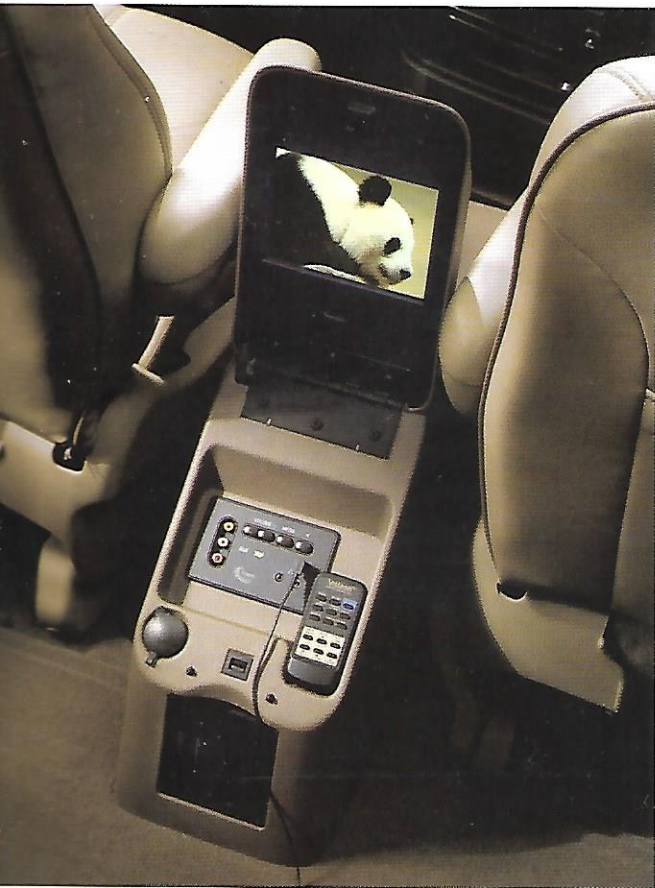
Optional Visteon Rear Seat Entertainment System includes a 6.4-inch screen, VHS player with infrared remote control and Plug/Play capability for video games. Sound comes by way of speakers or two sets of rear seat headphones (included). Late availability.
