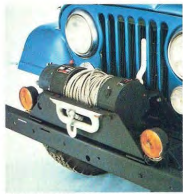
Electric winch—dealer installed
