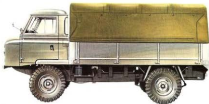
Truck-cab with fixed-side body and three-quarter length hood.
