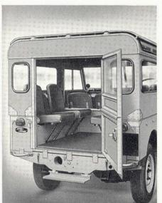
The rear compartment has plenty of room for four passengers on individual foam rubber tip-up seats. A wide rear door, opening from the side, and a folding step give easy access.
