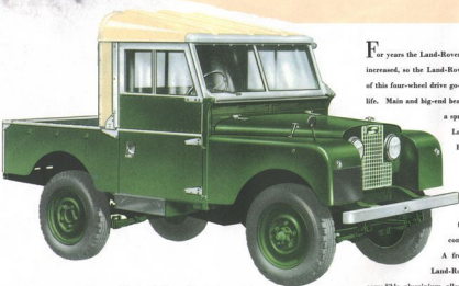
Above: The Land-Rover fitted with metal track cab (available at extra cost), providing an all-enclosed, weather-proof driving compartment and leaving the rear section open for ease of loading or unloading.
