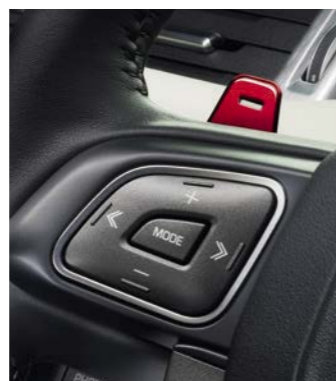
Gearshift Paddles VPLVS0187MMU – Aluminum VPLVS0187CAY – Red These Gearshift Paddles are machine polished, anodised and hand brushed to provide exceptional wear resistance with a premium finish.
