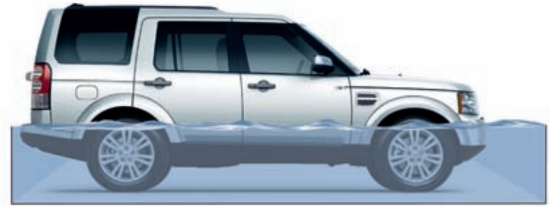
Wading Depth Maximum wading depth 27.56 in. (700mm) (with air suspension raised) Normal wading depth 23.62 in. (600mm)
