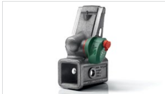
Quick Release Tow Hitch Receiver LR019990 Lockable for security. Easily removed. 1.9 inches/48mm Tow ball, height 15 inches/381mm from ground. 7,716lbs/3,500kg trailer load capacity (551lbs/250kg trailer nose load).
