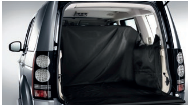
Flexible Loadspace Protector VPLAS0015 Heavy duty fabric helps protect loadspace up to window height. Also covers loadspace floor with second row seats folded. Includes heavy duty gloves.
