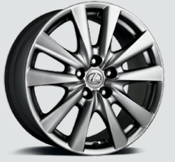
18-in split-five-spoke alloy wheels with Superchrome finish 1 AVAILABLE (BASE AND PREMIUM PACKAGE)
