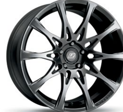
F SPORT 19-in full-face forged alloy wheels 2,3 AVAILABLE IS (RWD), IS C
