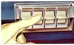
Lincoln Power Window Lifts let the driver control all four windows in the car by touching the switches ahead of the door panel. There's a separate control for each of the other three windows so that passengers can raise or lower the windows nearest them. (Standard equipment on Premiere models, extra cost option on Capris.)
