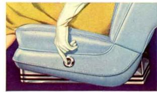
Lincoln Four-Way Power Seat has one switch, Just touch it and the seat moves up or down, backward or forward, until you're in the most comfortable driving position for you. This Lincoln "first" provides a completely individual, customized driving seat—and wonderful comfort. (Standard equipment on Premiere, extra-cost option on Capris.)
