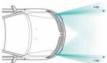
Available **adaptive HID headlamps** are truly illuminating. Based on steering wheel angle and vehicle speed, motorized low-beam projector headlamps turn in the same direction as MKZ – rotating 5° inboard and 15° outboard. This simple swivel action helps make more of the roadway visible around a curve.
