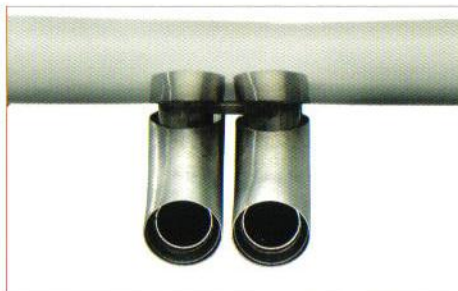
LOTAC05334: Level 1 Sports Exhaust (Elise/Exige 6 speed) (track use only) A compact silencer which offers visual and sound enhancement over the standard unit.
