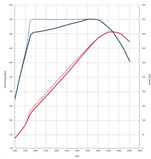
Two parallel-mounted, low-inertia turbochargers help prevent turbo lag, and give greater elasticity and faster response. In addition, the engine features highly innovative engineering solutions that have been developed to improve fuel efficiency: a high-pressure (200 bar) direct injection system and the adoption in both cylinder heads of two continuous phase timing variators which advance or delay the intake and exhaust valve timings. The driver can choose from three different
