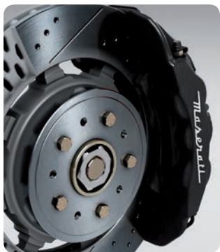
Brake callipers GranCabrio Sport painted Nero Drilled and slotted brake discs
