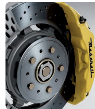
Brake callipers GranCabrio painted Giallo Drilled brake discs
