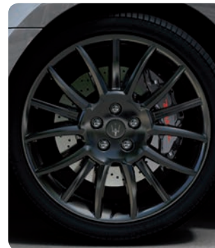
Alloy wheels Trident design Grigio Mercury (8,5J x 20" front; 10,5J x 20" rear)
