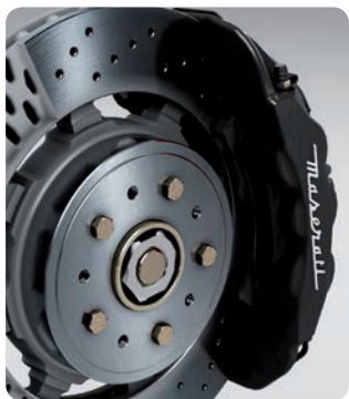
Brake callipers GranCabrio painted Nero Drilled brake discs
