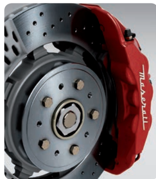
Brake callipers GranCabrio painted Rosso Drilled brake discs
