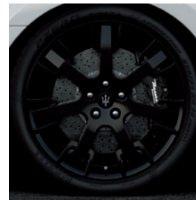
Brake callipers - painted Nero Alloy wheels - 20" Neptune Nero Lucido (8,5J x 20" front; 10,5J x 20" rear)
