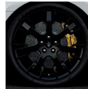
Brake callipers - painted Giallo Alloy wheels - 20" Neptune Nero Lucido (8,5J x 20" front; 10,5J x 20" rear)
