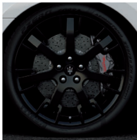
Brake callipers - painted Titanio Alloy wheels - 20" Neptune Nero Lucido (8,5J x 20" front; 10,5J x 20" rear)
