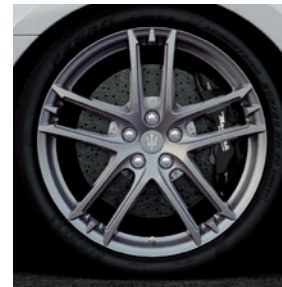
Brake callipers - painted Nero Alloy wheels - 20" MC-Design Titanio Lucido (8,5J x 20" front; 10,5J x 20" rear)
