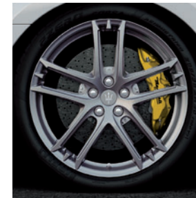
Brake callipers - painted Giallo Alloy wheels - 20" MC-Design Titanio Lucido (8,5J x 20" front; 10,5J x 20" rear)
