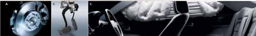
A. The power-assisted 4-wheel disc brakes on all MAZDA6 models also incorporate an Anti-lock Brake System (ABS) with Electronic Brakeforce Distribution (EBD) to help promote consistently linear, fade-resistant stops. B. The MAZDA6 utilizes a special brake pedal assembly that is engineered to fold away in the event of an accident to help minimize the chance of a serious ankle or leg injury. C. Advanced dual front air bags* are standard on all MAZDA6 models. Side-curtain air bags (with coverage for front and rear seats) and front seat side-impact air bags* are standard on most MAZDA6 models.
