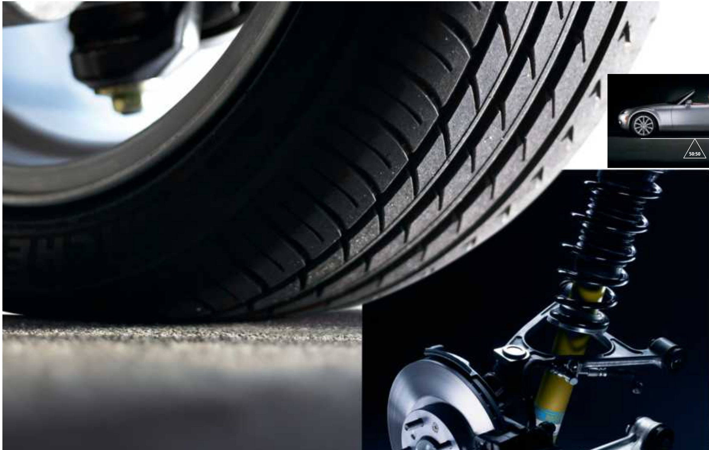
A. The MX-5 Miata's hollow front stabilizer bar helps reduce weight and minimize body roll while helping to maintain tire contact—especially during abrupt directional changes. B. An advanced double-wishbone front suspension, featuring aluminum alloy control arms and gas-filled shocks, helps promote quick response to all driver input and contributes to the MX-5 Miata's superb handling. Power-assisted ventilated front disc brakes with large 11.4-inch rotors promote consistently linear, fade-resistant stops.
