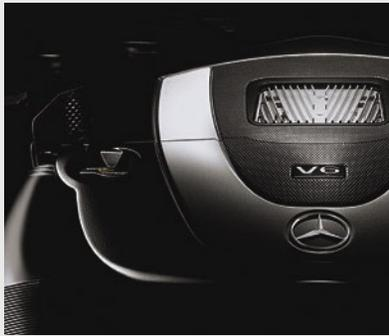
Pumping out 268 hp and 258 lb-ft of torque, the SLK 350's 24-valve DOHC V-6 features variable intake and exhaust valve timing, with continuously variable adjustment of all four cams up to 40° for smooth idling, rich midrange torque and high-rpm punch. Partnered with this is an innovative intake system engineered with movable "turbulence flaps" that vary the path and flow rate
