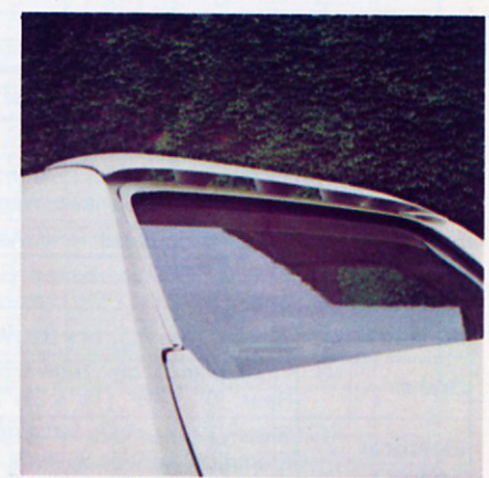
Opt. air deflector helps clear rear window.
