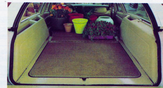
Carpeted rear cargo deck has 86.8 cu. ft. of load space for 4' x 8' materials with doorgate closed.
