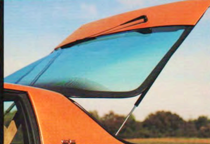
A rear hatch washer/wiper is standard on the S/E and available on Trans Am and Firebird.
