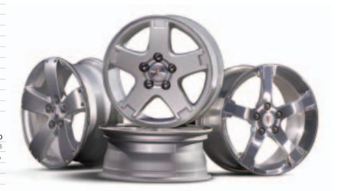
Left to right: Available 17" N75 cast aluminum flangeless wheel, standard 16" PYO cast aluminum wheel, available dealer-installed 17" forged aluminum flangeless wheel with polished finish.
