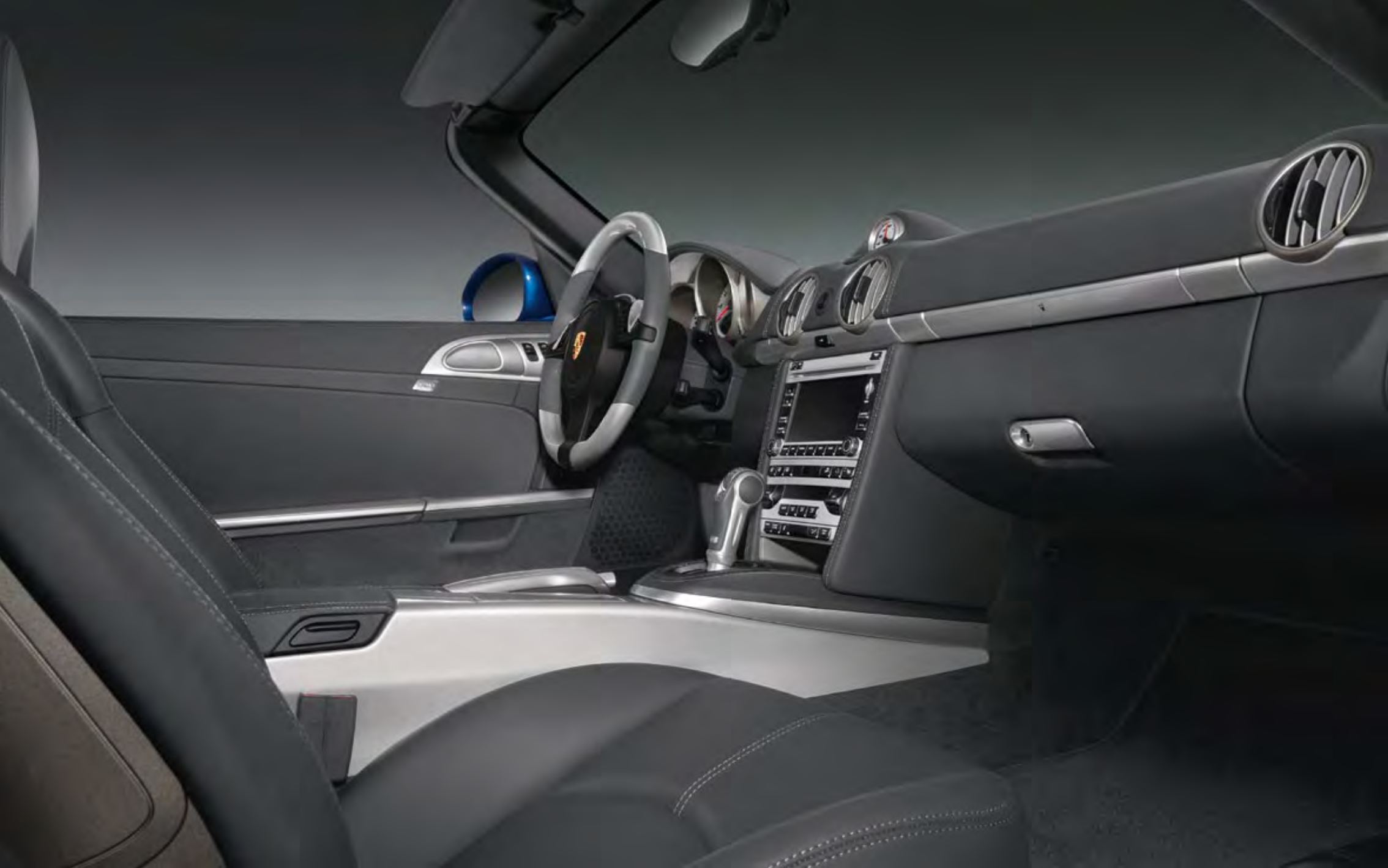
Ext ended trim package, three-spoke multifunction steering wheel, air vent slats, PCM package, and rear centre console in Aluminium Look; PDK gear selector and handbrake lever in aluminium; steering column casing and seat belt buckles in leather
