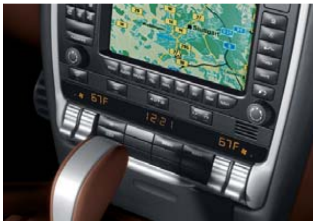
Air-conditioning control panel (cover open) below PCM
