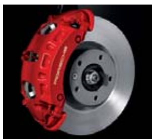
Cayenne Turbo: standard front brake with 14.49-in. disc
