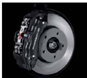
Cayenne: standard front brake with 12.99-in. disc
