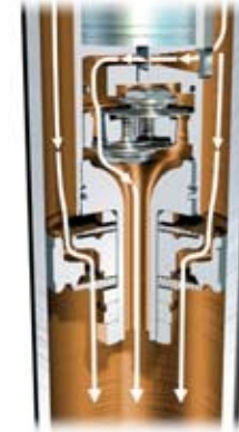
Rebound in ‘Normal’ mode – damper piston with bypass valve open
