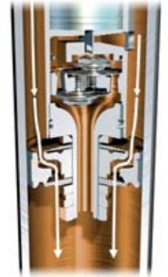
Rebound in ‘Sport’ mode – damper piston with bypass valve closed
