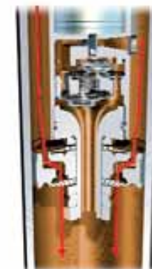
Rebound in 'Sport' mode – damper piston with bypass valve closed
