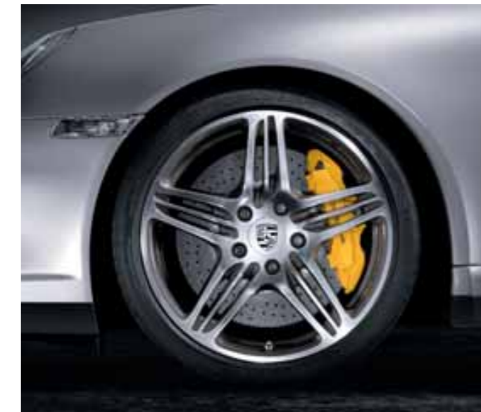
Porsche Ceramic Composite Brake (PCCB)
