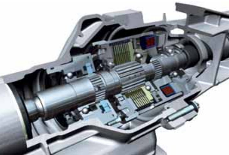
Electronically controlled multi-plate clutch
