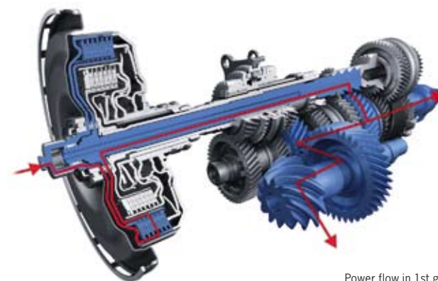
Power flow in 1st gear
